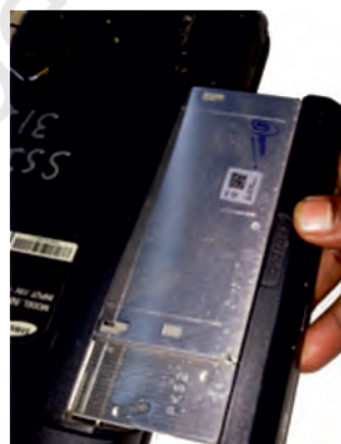
Fig. 12.67: Remove optical CD/DVD drive connector board
