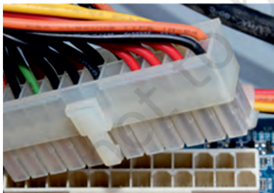
Fig. 12.45: Unplug 20-pin ATX
