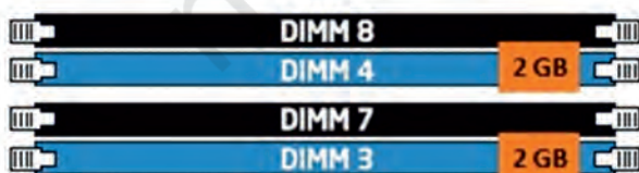
Fig. 9.11: Quad-channel with four DIMMs
