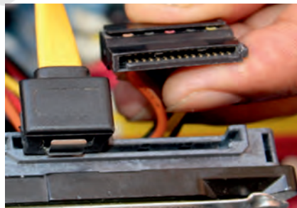
Fig. 12.40: Unplug 15-pin connector from HDD
