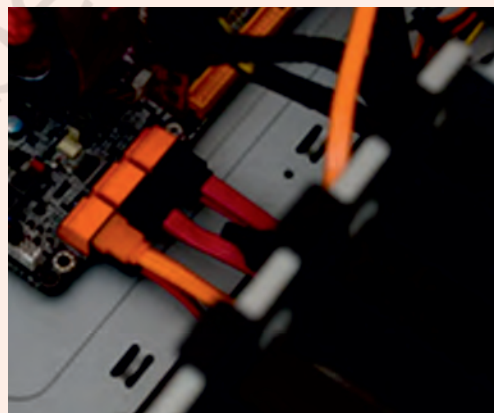
Fig. 4: Connect SATA data cable to the to optical drive motherboard
