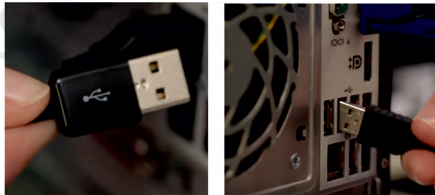
Fig. 12.24: Connecting keyboard in USB port
