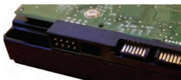
Fig. 10.12: Back of EIDE drive
