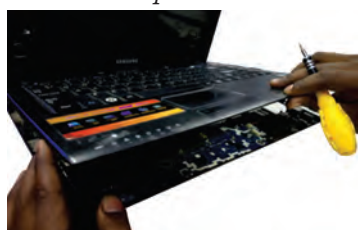
Fig. 12.60: Separate palm rest from bottom case
