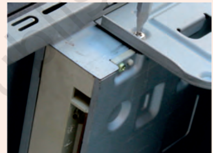
Fig. 2: Tighten screws of optical drive
