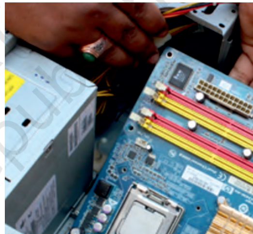
Fig. 12.55: Removing the motherboard
