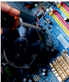
Fig. 12.8: Screw the heat sink fan assembly
