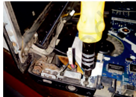
Fig. 12.70: Open the hinge and remove DC power jack
