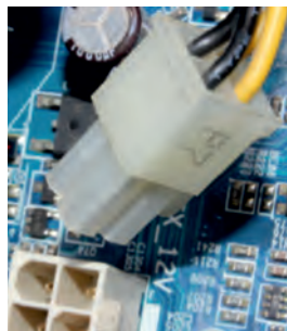
Fig. 12.46: Unplug 4-pin AUX power connector from power connector from motherboard
