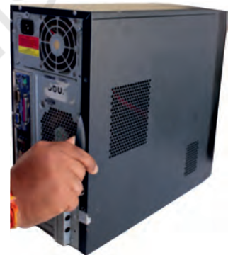
Fig. 12.39: Pull cabinet side cover
