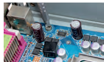
Fig. 12.11: Tighten all the motherboard screws
