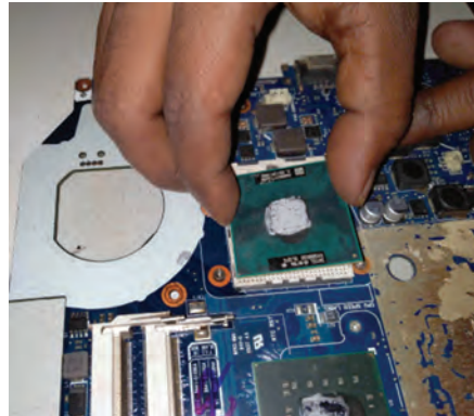
Fig. 12.58: Fit processor in the socket
