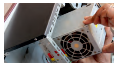
Fig. 12.4: Insert power supply
