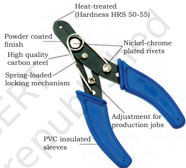
Fig.11.7: Wire stripper and its different parts
