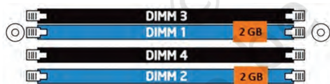
Fig. 9.9: Dual-channel with two DIMMs
