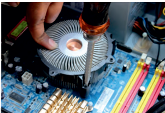
Fig. 12.44: Unscrew heat sink
