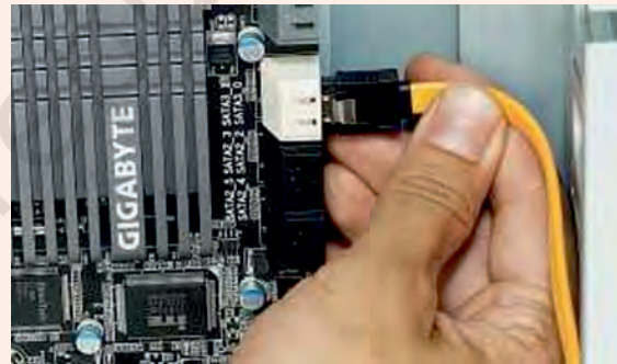
Fig. 6: Plugging SATA data cable into the motherboard
