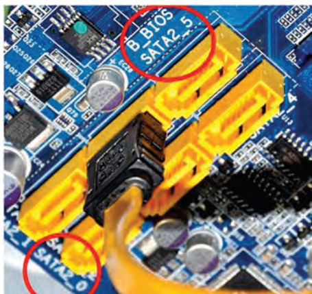
Fig. 10.14: SATA port in motherboard
