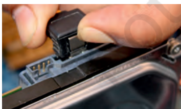
Fig. 12.16: Connect cable IN to HDD
