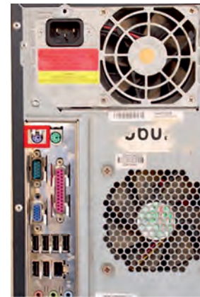
Fig. 12.25: Connecting mouse (a) in PS/2 port (b) in USB port
