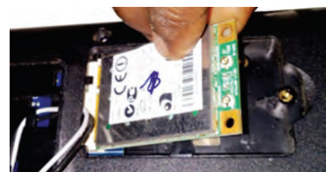
Fig. 12.72: Disconnect Wi-Fi Module
