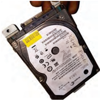
Fig. 12.63: Remove hard drive assembly
