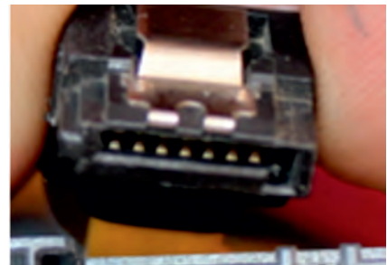
Fig. 12.41: Unplug 7-pin connector from HDD
