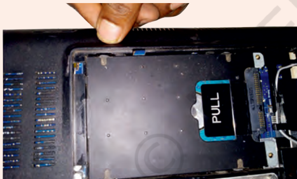
Fig. 3: Open connector and release hard drive cable
