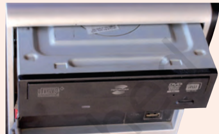
Fig. 1: Insert optical drive
