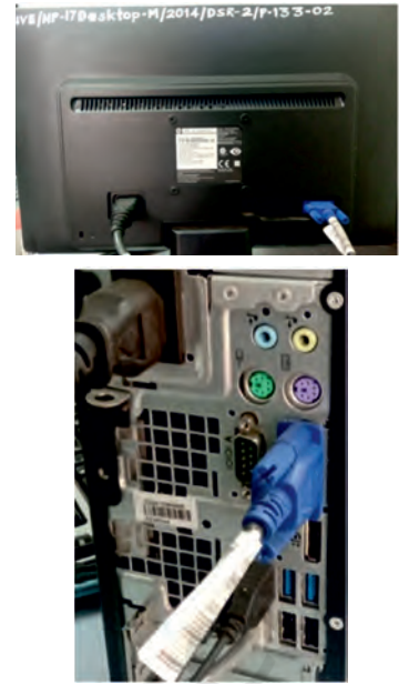
Fig. 12.30: Proper connectivity of parts of computer system
