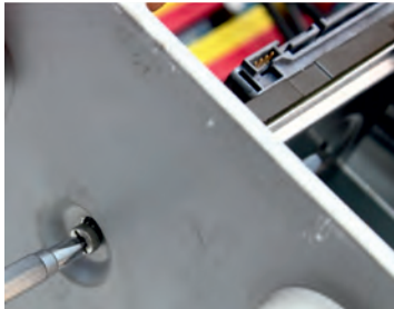
Fig. 12.13: Tighten screws of HDD
