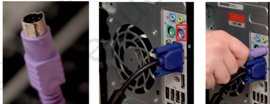
Fig. 12.23: Connecting keyboard in PS/2 port
