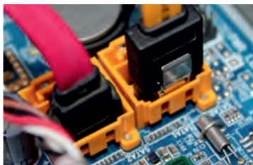
Fig. 12.47: Unplug SATA cables from motherboard
