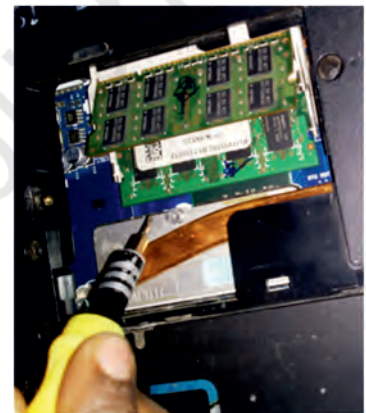
Fig. 12.65: Remove RAM memory modules
