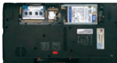
Fig. 12.61: Remove screws from the hard drive and disconnect it
