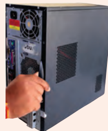
Fig. 2: Remove the side panel
