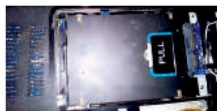
Fig. 12.62: Open the connector and release hard drive cable
