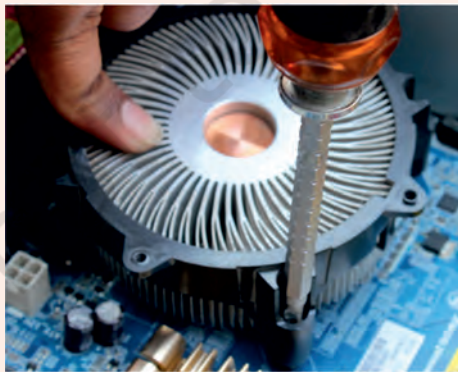
Fig. 1: Screwing the heat sink
