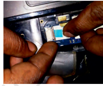
Fig. 12.75: Keyboard permanently attached to top case
