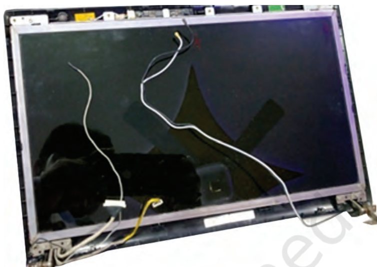
Fig. 12.79: Separate LCD screen from back cover
