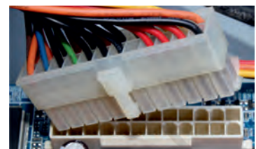
Fig. 12.18: Plug-in 20-pin ATX power connector to motherboard
