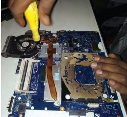
Fig. 12.57: Unscrew the socket
