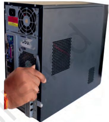
Fig. 12.2: Pull cabinet side cover
