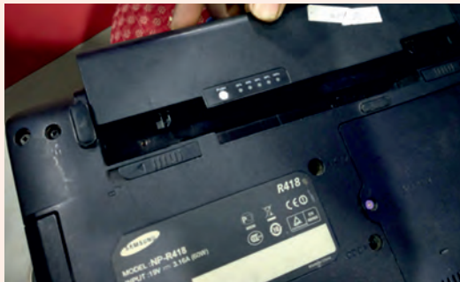
Fig. 1: Remove battery and optical drive
