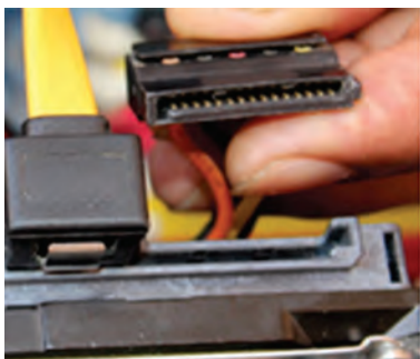
Fig. 12.48: Unplug power cable from optical drive and HDD
