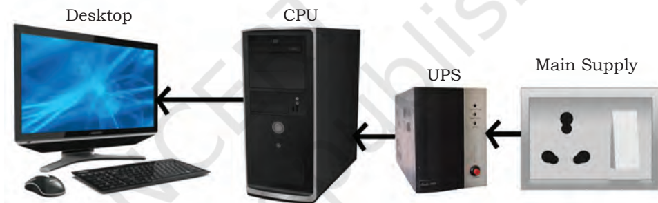
Fig. 12.29: Power connection (CPU through UPS)
