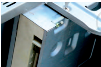
Fig. 12.15: Tighten screws of optical drive
