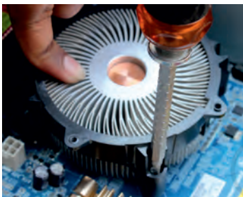
Fig. 12.7: Screw the heat sink
