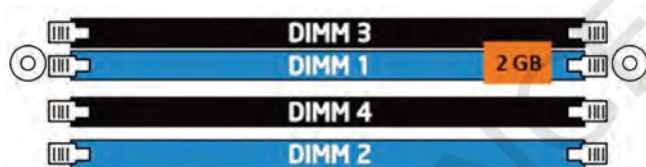
Fig. 9.8: Single-channel with one DIMM
