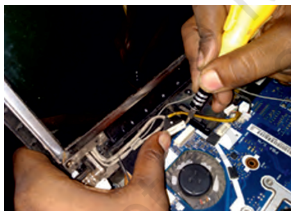
Fig. 12.80: Disconnect video cable from screen
