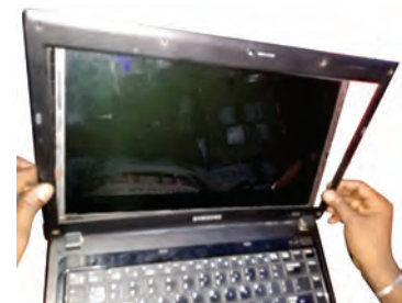
Fig. 12.76: Notebook PC LCD screen removal
