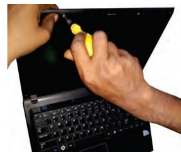
Fig. 12.77: Remove the four screws securing LCD screen
