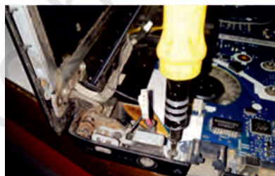
Fig. 12.71: DC power jack mounted under display hinge
