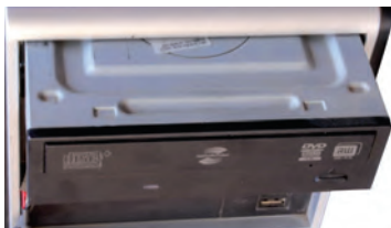
Fig. 12.14: Insert optical drive
