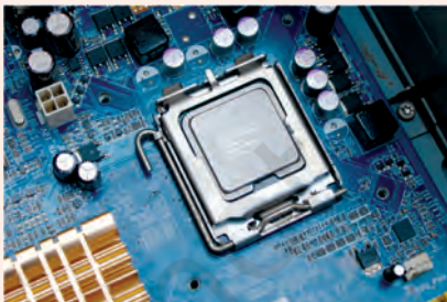
Fig. 1: Installing CPU on the motherboard
