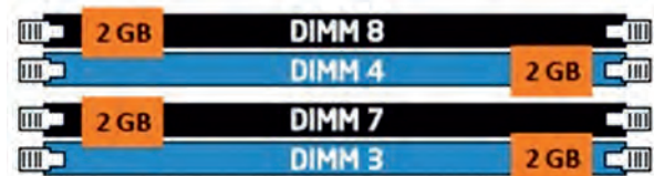
Fig. 9.12: Quad-channel with eight DIMMs
