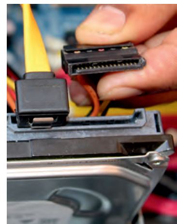
Fig. 12.20: Plug-in 15-pin connector to HDD
