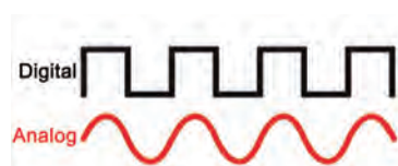
Fig. 2.9: Digital and analog signals
