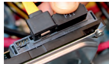
Fig. 12.17: Press cable socket for proper connection
