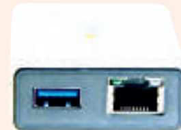
Fig. 4: RJ-45 Ethernet port to connect HDD
