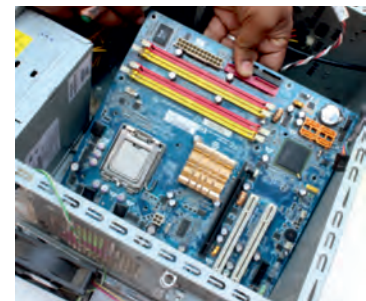
Fig. 12.10: Lay the motherboard over the standoffs
