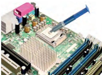
Fig. 12.6: Applying thermal compound on CPU
